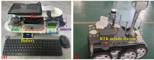
Fig. 4. Datasets are collected on two platforms. (a) A handheld device. (b) A mobile vehicle.
