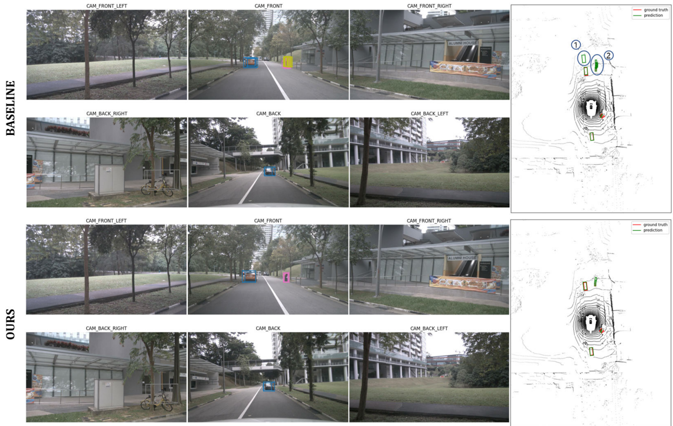
FIGURE 4. Visualization of detection results on the nuScenes dataset, comparing the BEVDepth [1] baseline with our proposed method. Predicted 3D bounding boxes are shown in the camera views using class-specific colors: blue for car, gray for bicycle, yellow for pedestrian, and pink for motorcycle. On the BEV maps, predicted boxes are shown in green and ground-truth boxes in red. Numbered circles indicate key differences.
