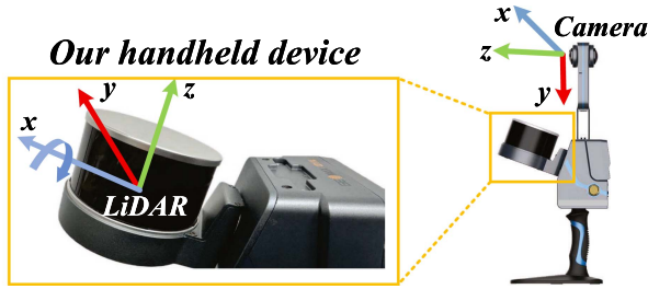
Fig. 9. Our mobile mapping system. It consists of a Velodyne VLP-16 LiDAR mounted on motor platform and an omnidirectional camera.
