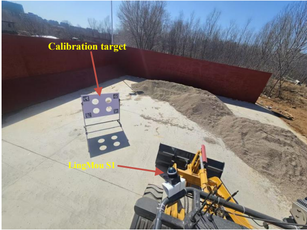
Fig. 5: Actual experimental scene of LiDAR-dual-camera extrinsic calibration on a wheel loader
