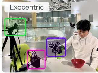
Fig. 2: Left: DexWild efficiently capture high-fidelity data using an individual’s own hands across various environments. Right: Robot hands are equipped with cameras aligned with the human cameras. We test DexWild on two distinct robot hands and robot arms.
