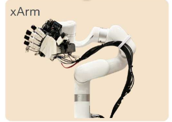
Fig. 2: Left: DexWild efficiently capture high-fidelity data using an individual’s own hands across various environments. Right: Robot hands are equipped with cameras aligned with the human cameras. We test DexWild on two distinct robot hands and robot arms.
