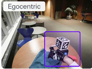
Fig. 2: Left: DexWild efficiently capture high-fidelity data using an individual’s own hands across various environments. Right: Robot hands are equipped with cameras aligned with the human cameras. We test DexWild on two distinct robot hands and robot arms.
