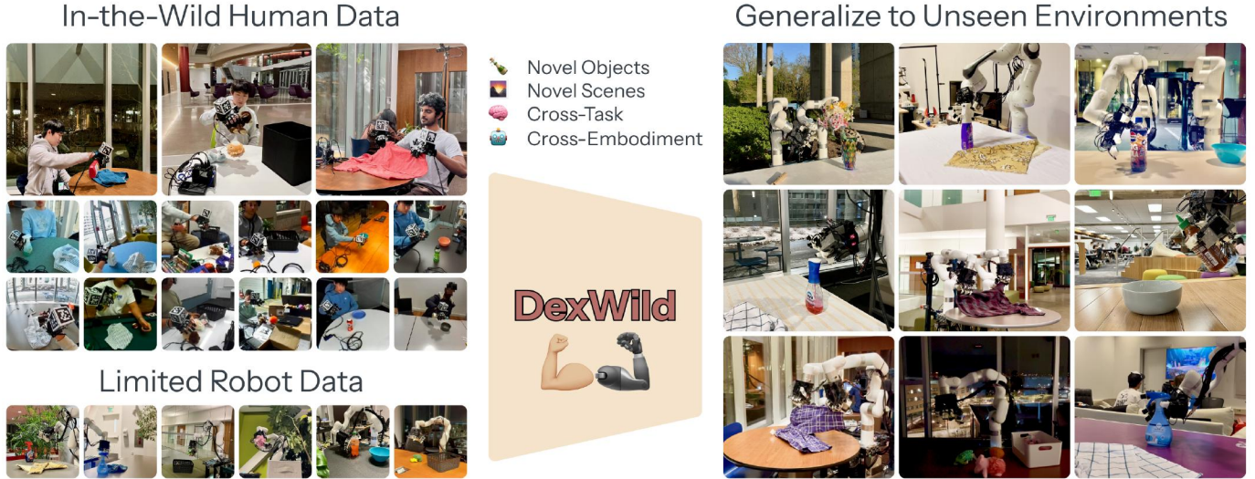
Fig. 1: DexWild enables dexterous policies to generalize to new objects, scenes, and embodiments. This is achieved by leveraging large-scale, real-world human embodiment data collected in many scenes and co-trained with a smaller robot embodiment dataset for grounding.
