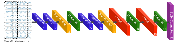
Fig. 2. ConVLSTM: the DL architecture used for processing wearable and force/torque sensor data.
