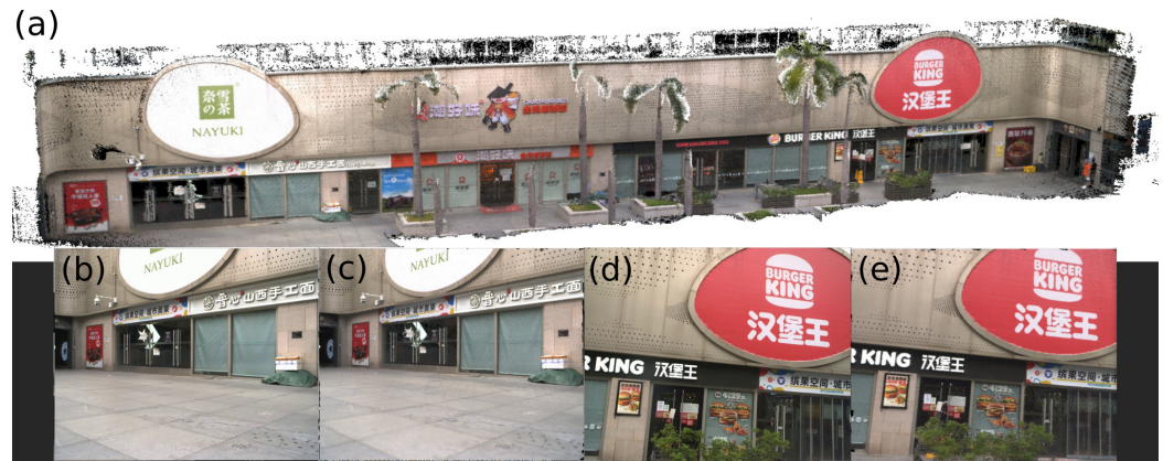
Figure 1. Retail Street sequence. (a) Three-dimensional reconstruction of the Retail Street sequence obtained with FastLivo2. (b,c) Real image and its corresponding image rendered from the point cloud. (d,e) Real image and its corresponding image rendered from the point cloud.
