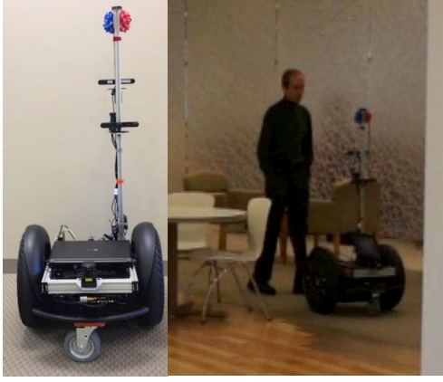
Figure 2. (left) The blind aid robot, a mobile platform with the ability to track people and investigate the environment. (Right) A person following the blind-aid robot through an indoor setting.
