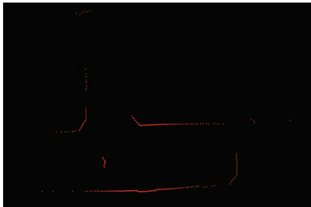
Fig. 3. Example of pointcloud data from 2D-LiDAR
