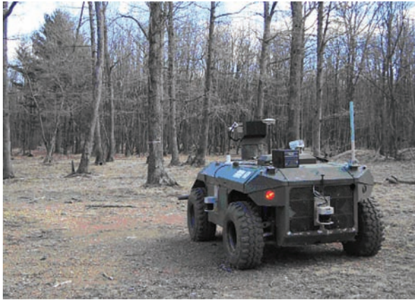
Fig. 1. The Demo III Experimental Unmanned Vehicle (named XUV) used in our tests. The vehicle shown is equipped with a 3D LADAR mounted on a pan-tilt platform.
