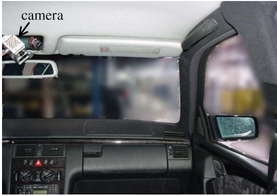
Fig. 2. Test vehicle equipped with a prototype camera mounted in the overhead module; the camera is able to survey the complete passenger seat.
