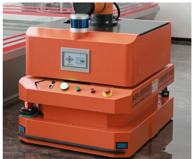
Fig. 11 Robot platform with LiDAR
