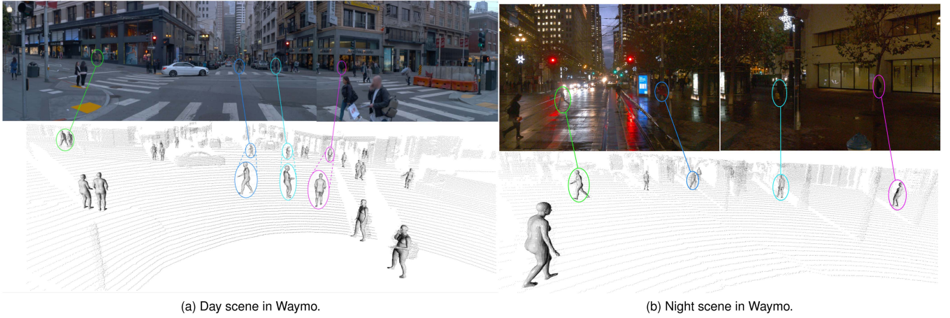
Fig. 3. Example results of LiDAR-HMR on multiperson scenes in the Waymo [36] dataset. RGB images are not utilized in the algorithm but they are illustrated for better visualization. LiDAR-HMR can reconstruct accurate human meshes under different illumination conditions.
