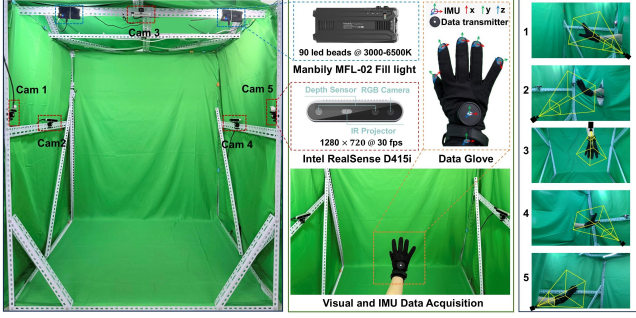
Figure 2: Recording setup with 5 temporally synchronized RGB-D cameras and a dataglove intergrated 7 IMUs.
