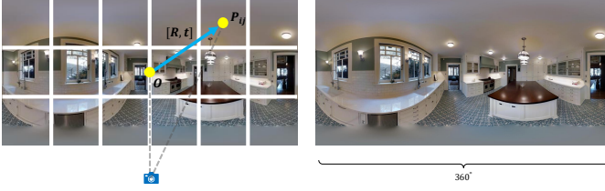
Fig. 3: Panoramic front-view generation in the Matterport3D dataset. For each center point P_{ij} of the narrow-view images, rotation R and translation t relative to a reference center O are used to construct the panoramic front-view image.
