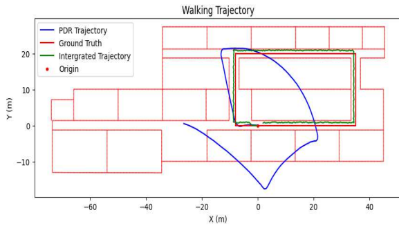
Fig. 6. Comparison of the trajectories of PDR only and NDT integrated PDR
