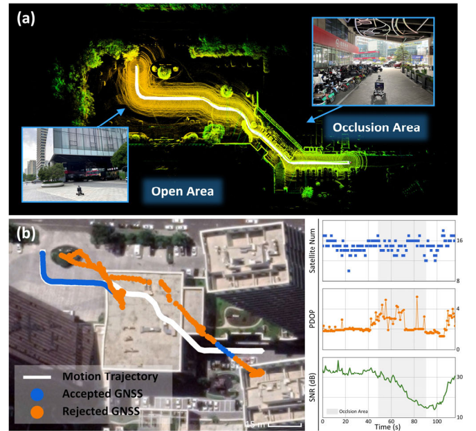
Fig. 13. Experiment in GNSS degraded scene (the bottom right panel is the corresponding status of available satellites). (a) Estimated trajectory and mapping results. (b) Utilization of GNSS measurements in the world frame.
