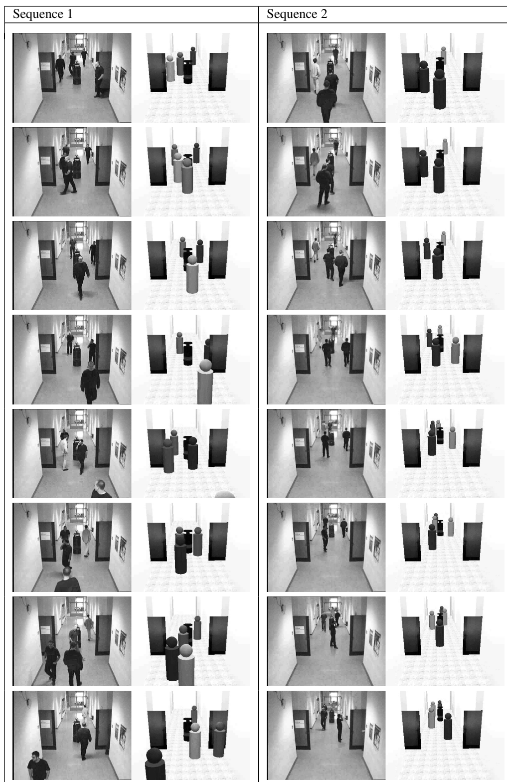
Fig. 5. Two short tracking sequences showing a real photo and a 3D visualization of the state estimate at the same point in time. The time delay between consecutive images is 1.25 s.
