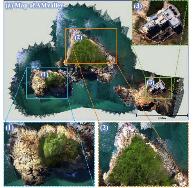
Fig. 6. Our large-scale mapping result in the MARS-LVIG HKisland01 dataset. The enlarged details show that the reconstructed RGB point cloud is dense, consistent, and maintains an accurate metric scale.
