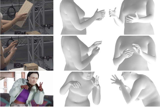
Fig. 7. Visualization of hands by SMPLeSt-X. SMPLeSt-X demonstrates robust hand pose estimation in whole-body pose and shape estimation tasks across various scenarios, including occlusion (top), object interaction (middle), and challenging hand poses (bottom).
