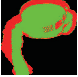
Figure 6. Example of pixel states by analyzing with PSA. Green, red and black pixels indicate stationary, transient and background states, respectively.
