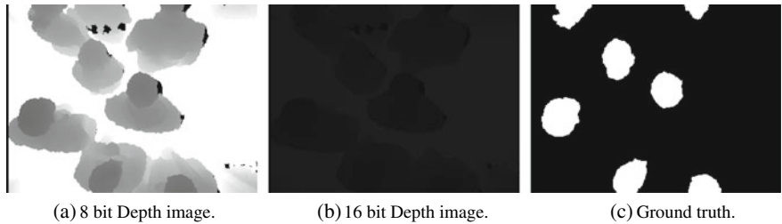
Fig. 18.14 TVHeads dataset. It consists of 8-bit scaled depth images (a), 16-bit original images (b) and the corresponding ground truth (c) [33]
